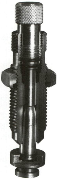
Figure 28 Cutaway of Bullet Seating Die
