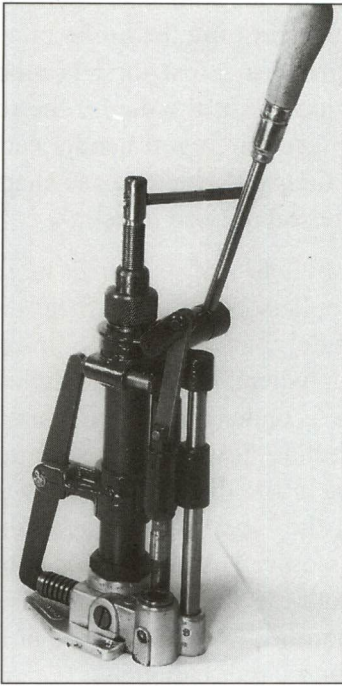
Figure 48 Star lubricator and sizer. Bullets are pushed through the die and drop out of the bottom
